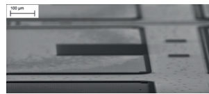
SEM image of partially processed MOSFETs
